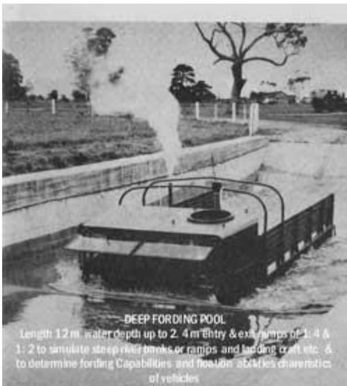
**Deep Fording Pool:** Length, 12m. Water Depth, up to 2.4 meters. Entry and exit ramps of 1:4 and 1:2 to simulate steep river banks or ramps on landing craft etc. This is used to determin fording capabilities and flotation abilities and characteristics of vehicles.
