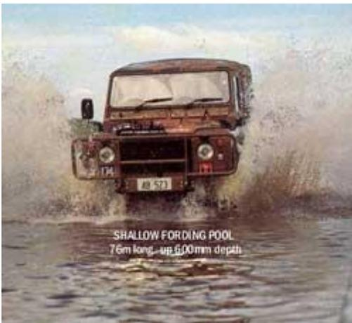
**Shallow Fording Pool:** 76 meters long and up to 600mm in depth.
