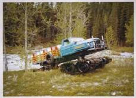
In 1955, Bruce's invention of the double sprocket made it possible to drive wide tracks and also keep them in place while using a single row of wheels. The combination of the splice in the belt and the double sprocket allowed the use of any size or shape belt the vehicles needed. The "wide track" concept was born. They were now able to build a new and different type of machine.
