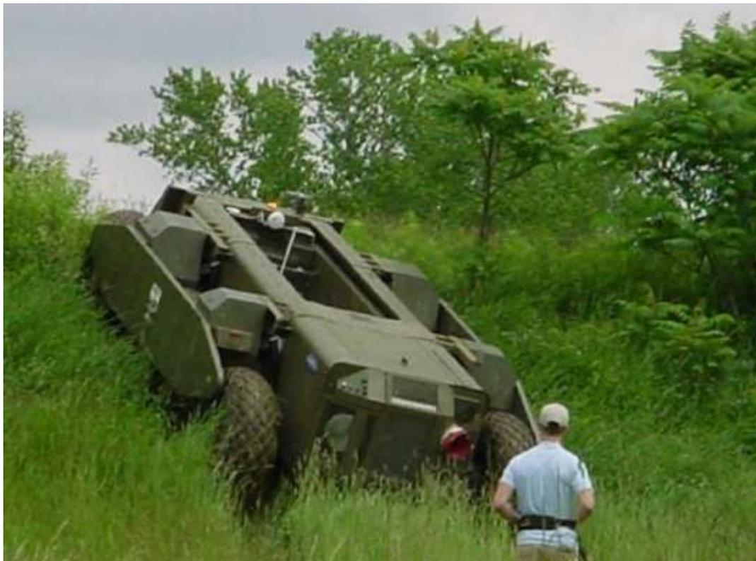
Team Spinner rolled out its seven ton version on 06 February 2003 in Pittsburgh, Pa. The Team Spinner UGCV will carry an assortment of payloads weighing approximately 4,500 pounds and is close to the size of the Future Combat Systems' Armed Reconnaissance Vehicle. Team Spinner, lead by Carnegie Mellon University, includes team members Boeing, Timoney Technology, and PEI Electronics Inc.
